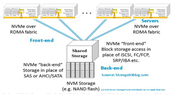
Various NVMe front-end including NVMeoF along with NVMe back-end devices (<u>U.2, M.2, AiC</u>)
