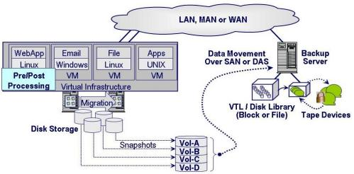
Figure-3: Proxy-Based Backup Such as VMware VCB
