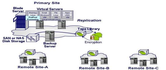
Figure-1: Providing High Availability and Protecting Local and Remote Virtual and Physical Servers
