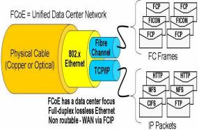
Figure-3 Common cabling separate networks
